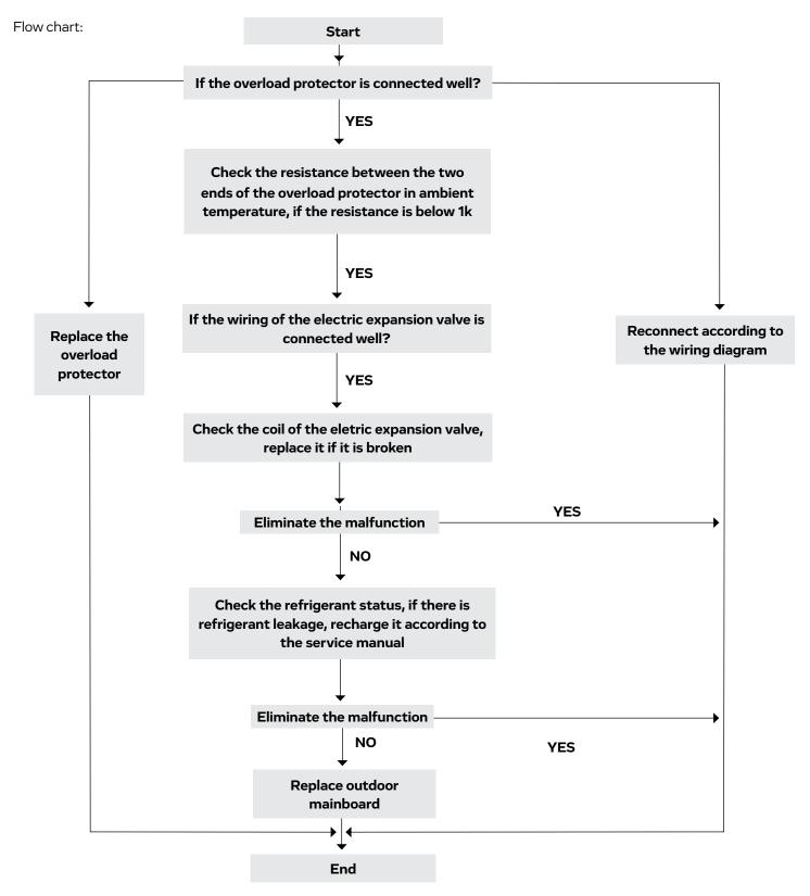
Note: the detection method of the coil of the eletric expansion valve: there is five pieces of coil of the eletric expansion valve, the resistance of one of them (the leftmost or the rightmost one) is almost the same as the resistance of other terminal (within  $100\Omega$ ). Judge the condition of the electronic expansion valve through detecting these resistance.
