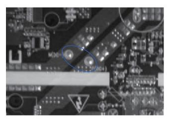
1 IPM protection malfunction: Main checking point:
